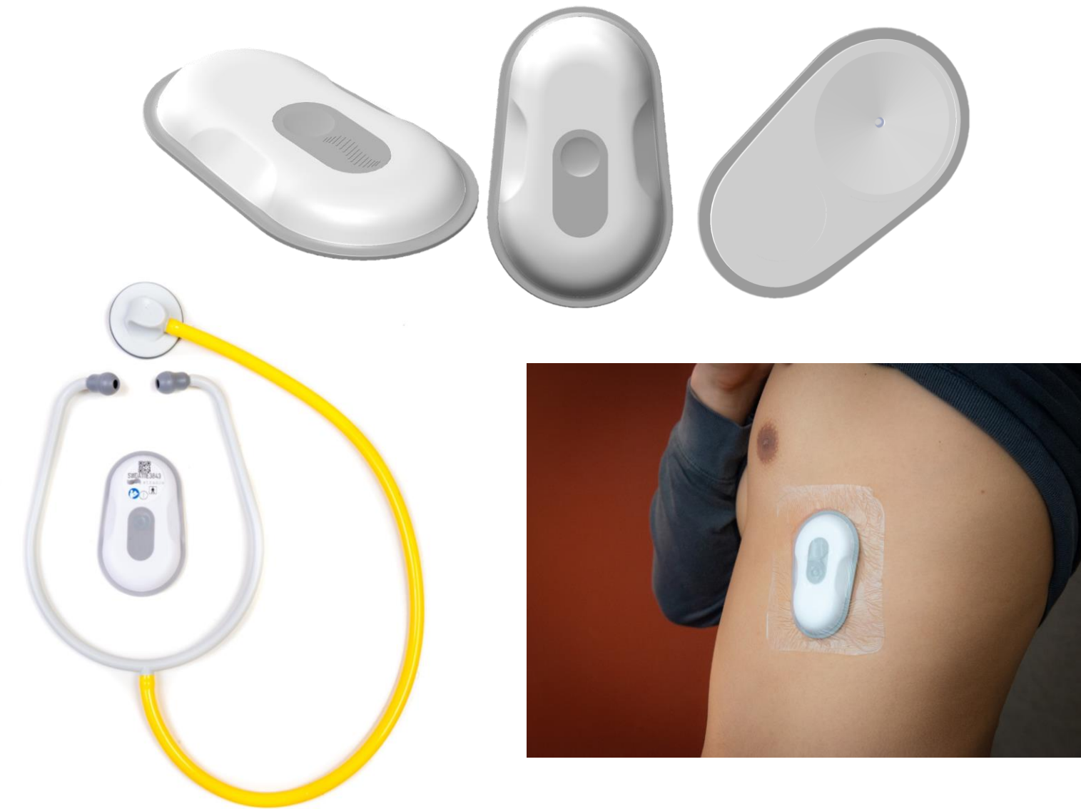
Figure 1. The SWD passively detects, amplifies, collects, and stores lung sounds. The SWD is rechargeable and has 10-24hr of battery life depending on configuration. It was designed to be cleaned with commonly used antiseptic wipes.
